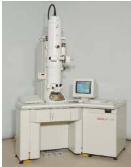
Figure 4.9 Transmission electron microscope (TEM)
